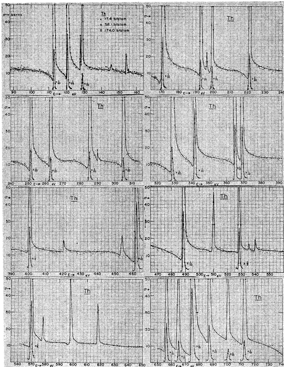
FIG. 1. The "measured" total neutron cross section of \text{Th}^{232} versus neutron energy. The peak values at resonances are limited by Doppler level broadening, experimental energy resolution, and the size of the 1/n value for our thinnest sample. Areas under these curves for the resonances may be quite different from the area under a true \sigma versus E plot.
